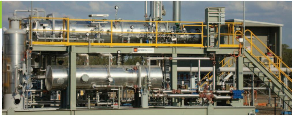
Dehydrated gas flows out of the top of the Contactor, while the Rich Glycol flows out of the bottom of the Contactor and to the Glycol Regeneration Package.
