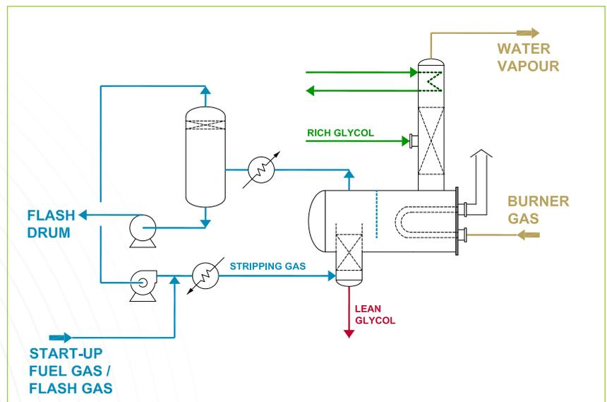
Patented GLYNOXX® closed-loop process – basic process shown in blue
