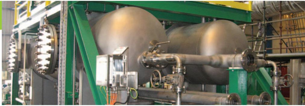
This recycled water stream is then returned to the IGF Vessel at selected entry points, where the gas bubbles are utilised for flotation of oil and fine solids from the oily water stream.
