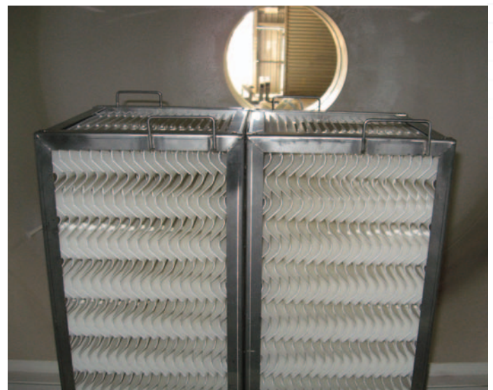
Pressurised CPI CAD Model (top) & CPI vessel internals (bottom)
