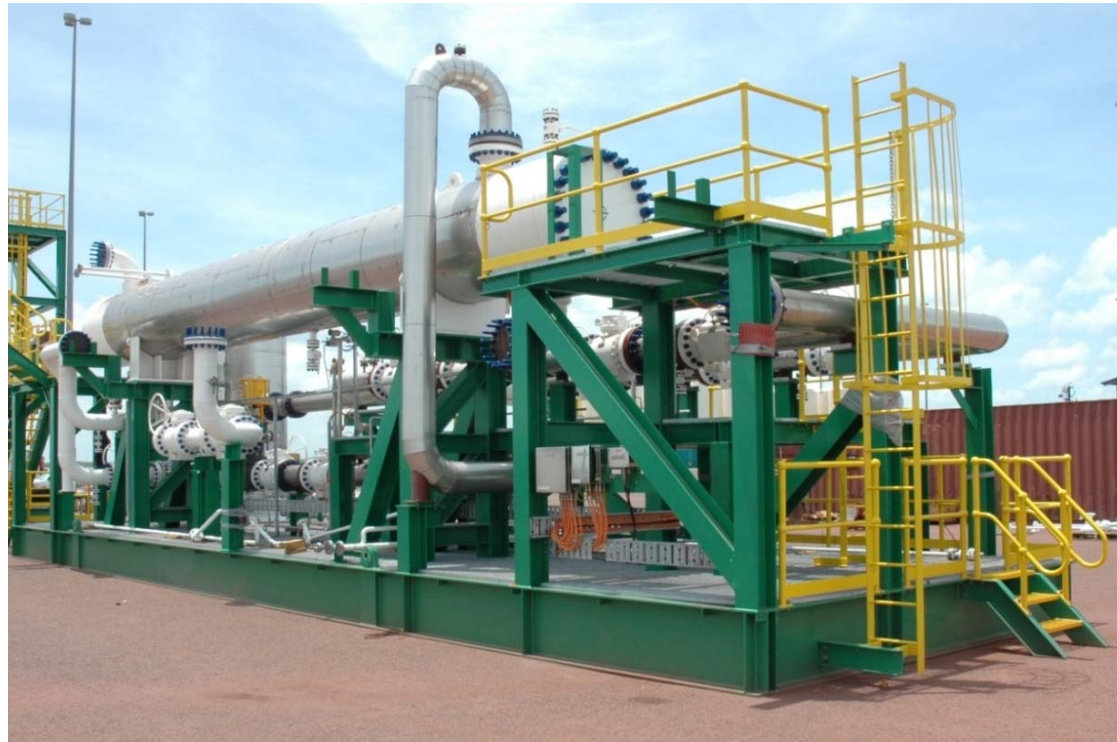
Image of ENI Blacktip Dew Point Control Unit during delivery, Northern Territory 2009
