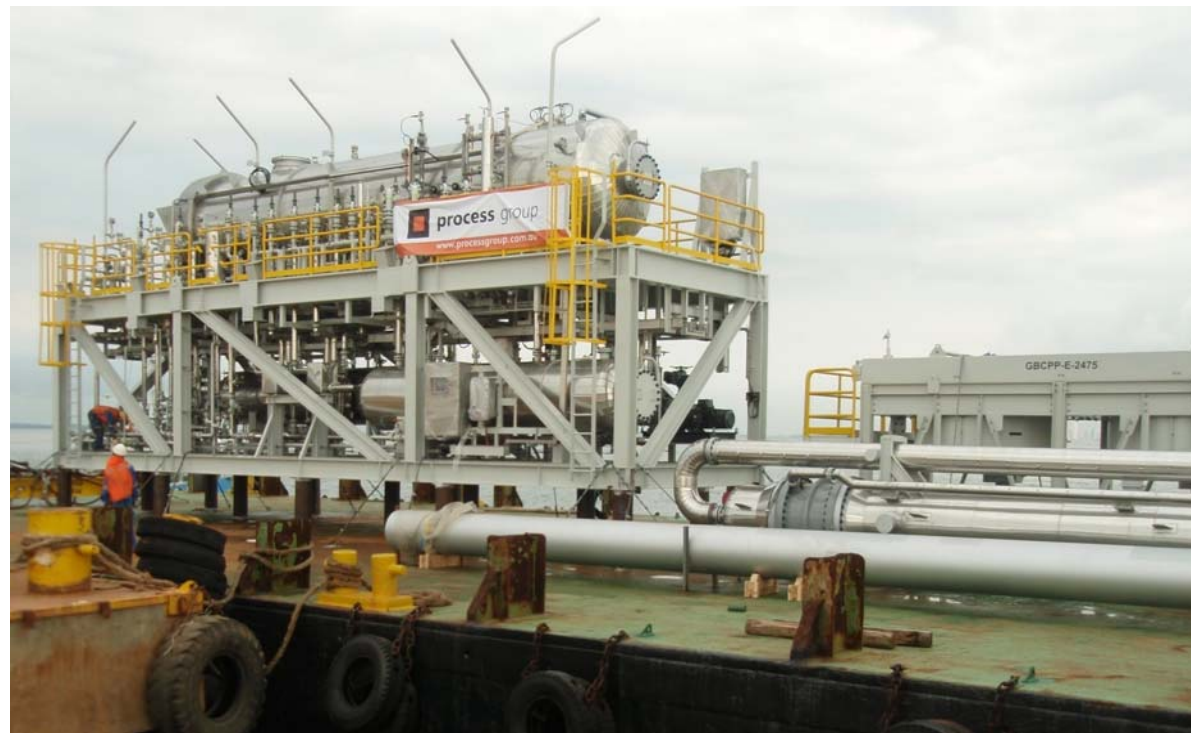
MEG Regeneration Package being prepared for delivery from Batam works', Indonesia.
