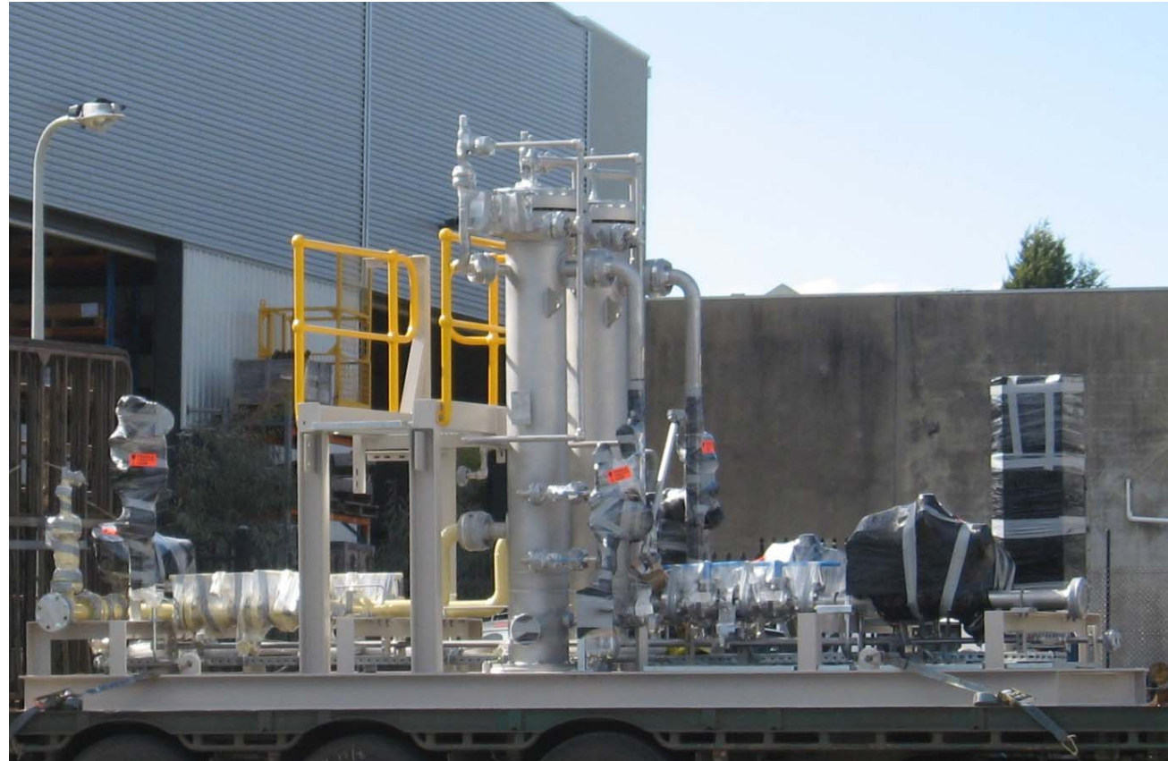
Fuel Gas Filter Skid ready for delivery at Process Group's workshop, Australia 2012.
