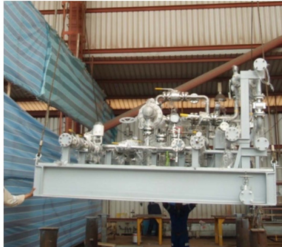
Deoiler Hydrocyclone skid nearing completion at Batam works, Indonesia 2010.
