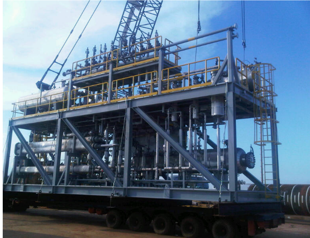
TEG Dehydration package being delivered from Batam works', Indonesia 2010
