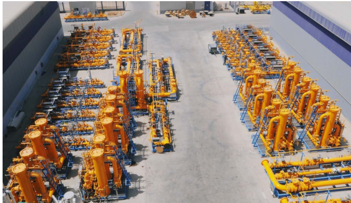
Filter Vessels and Gas Metering skids ready for delivery at Process Group International's workshop, 2008.
