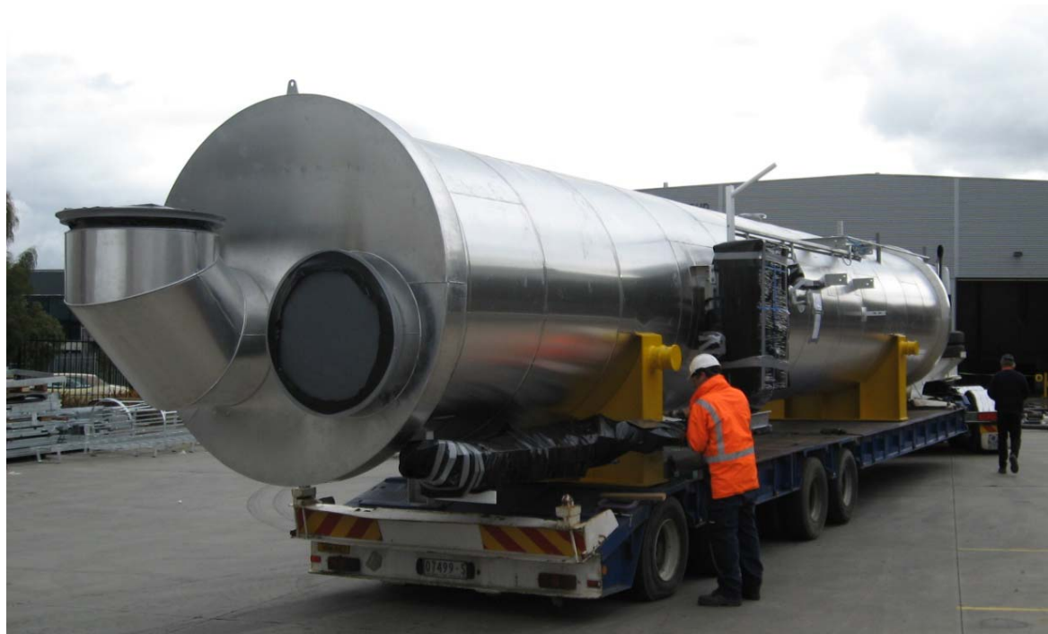
Water Bath Heater ready for delivery at Process Group's workshop, Australia 2012.
