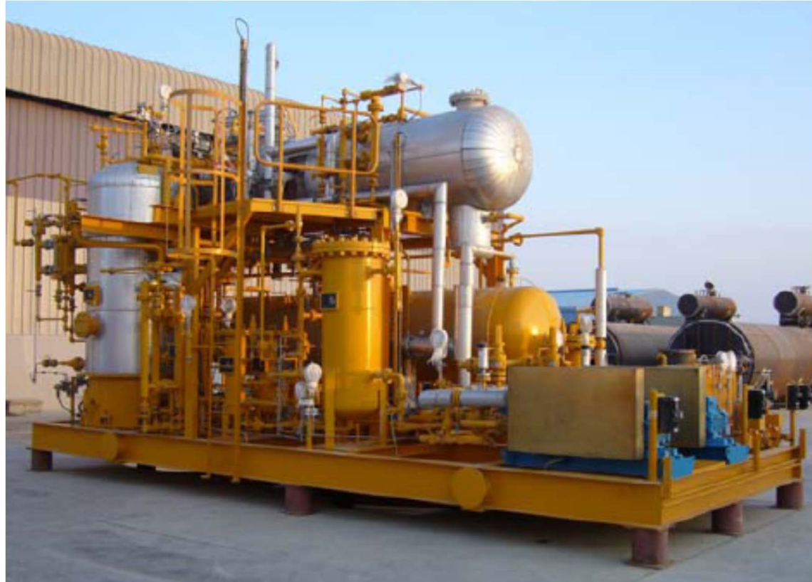
Bahregansar TEG regeneration skid ready for delivery from Process Group International's works, Abu Dhabi 2006
