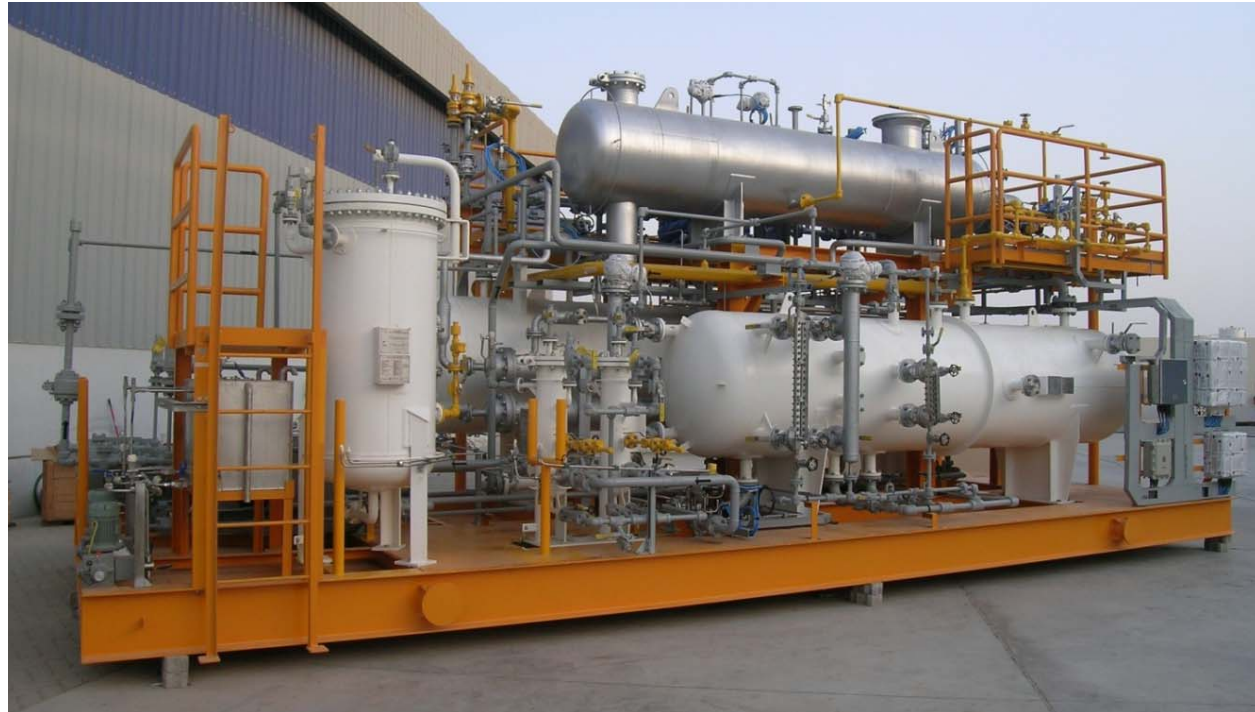
ICP-R TEG regeneration skid ready for delivery from Process Group International's works, Abu Dhabi 2010
