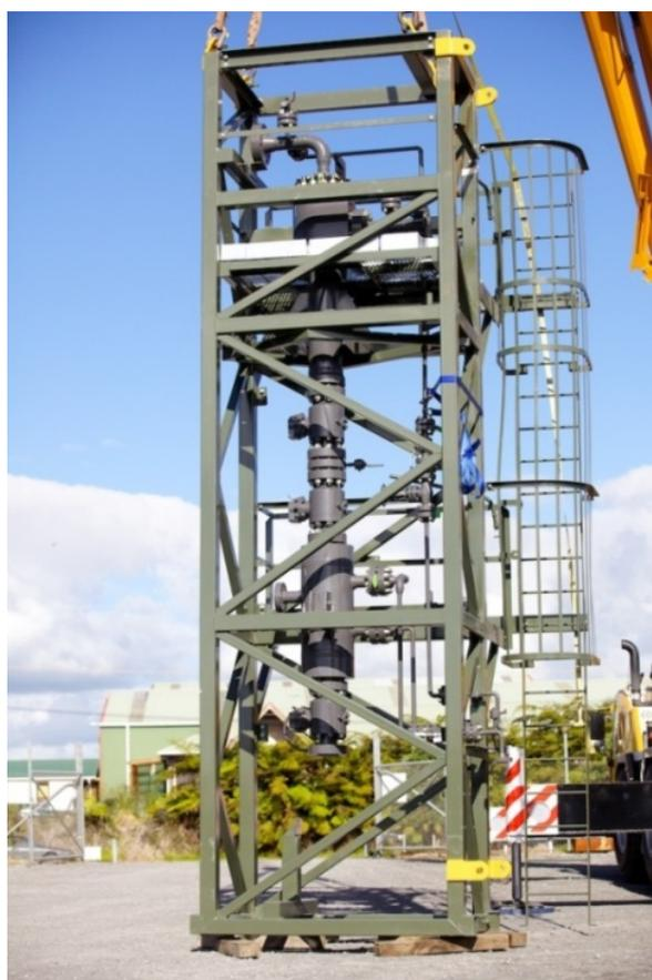
Figure 3: Completed well head desander package
