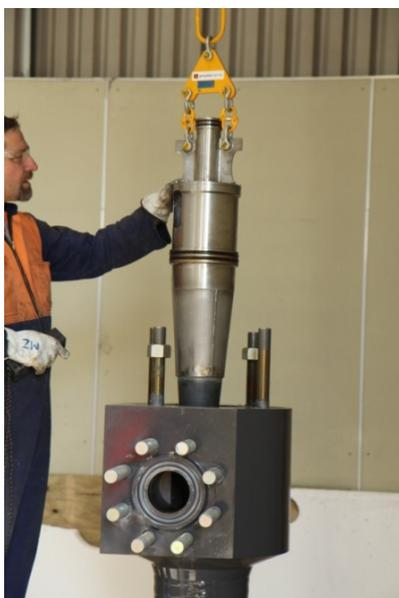
Figure 1: Desander cyclone being lowered into containment vessel.
