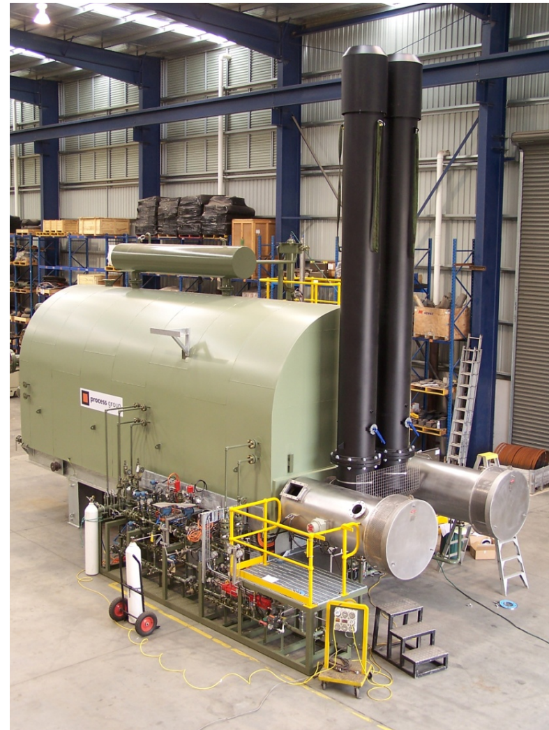
View of assembled Water Bath Heater at Process Group's workshop, 2010.
