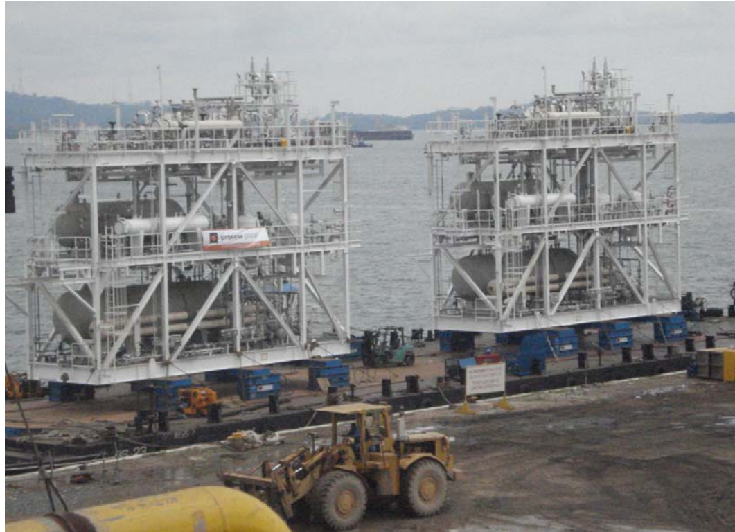
Two TEG Dehydration packages nearing completion at Batam works', Indonesia 2010
