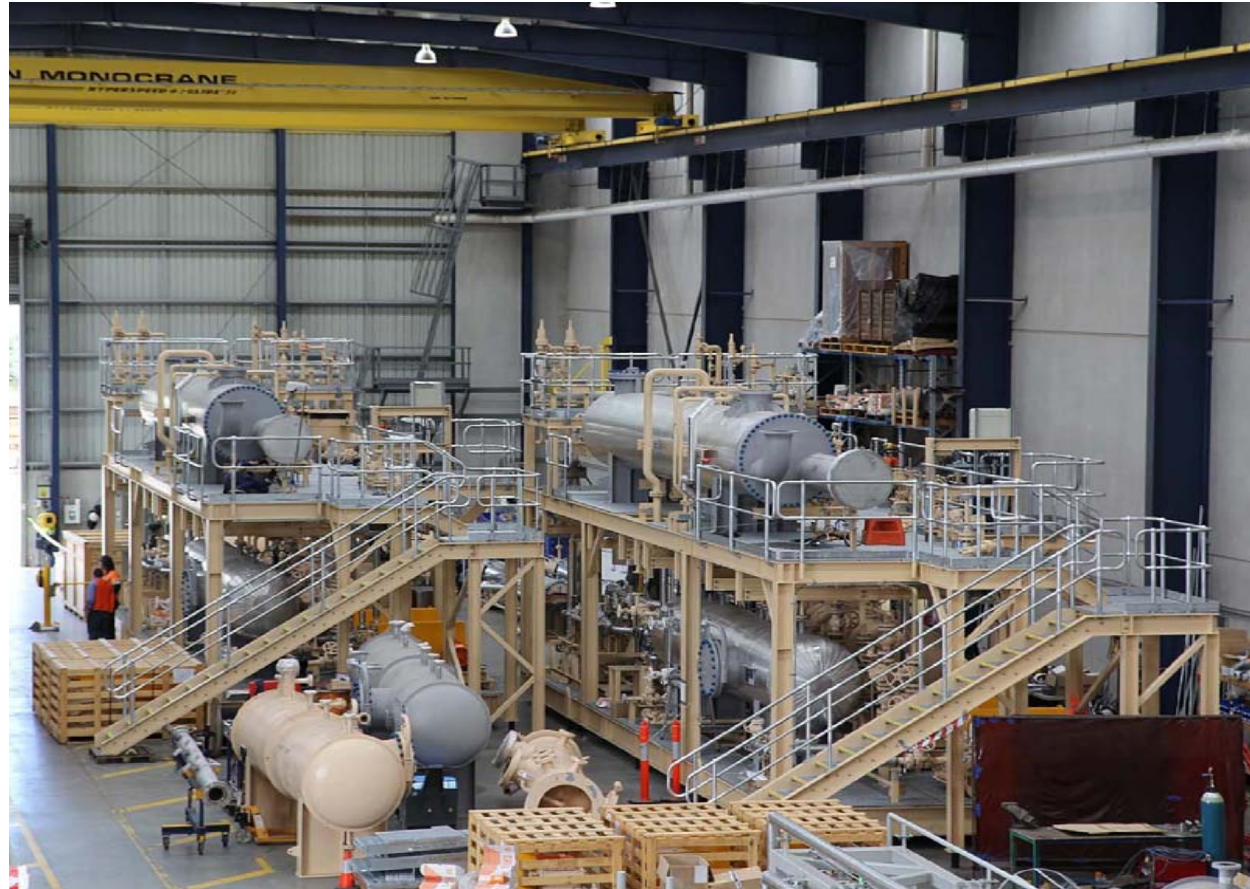
Two TEG Dehydration packages nearing completion at Process Group's works, Rowville 2012
