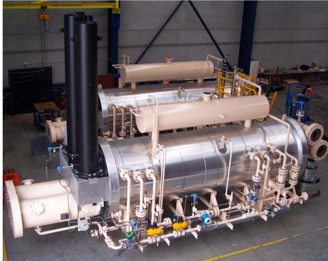
Assembled Water Bath Heaters at Process Group's workshop, 2010. From front to back; PH-GR and Pickanjinie.
