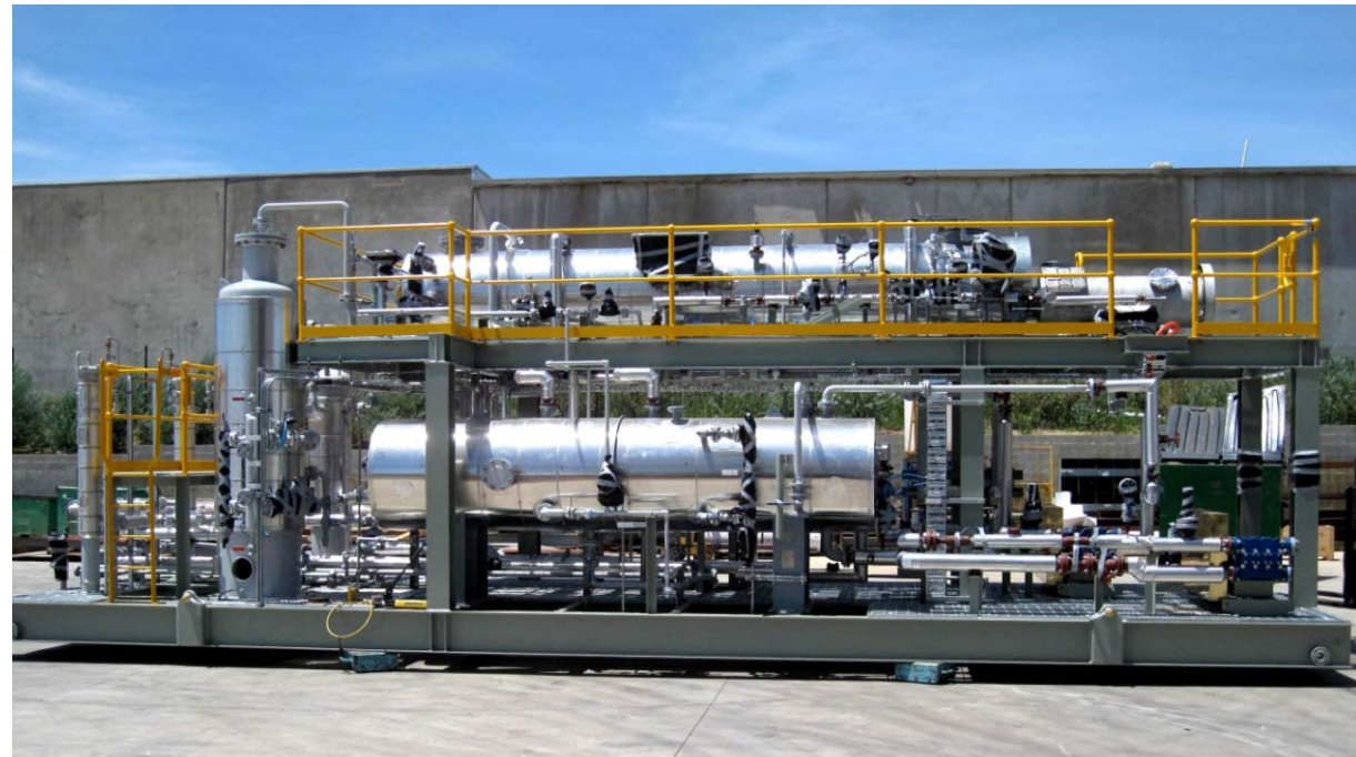
TEG Regeneration skid being prepared for delivery at Process Group's works, Rowville 2009.
