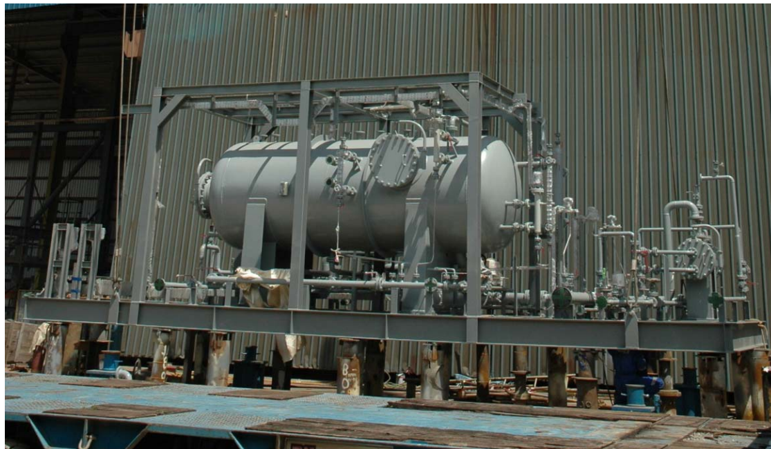
Induced Gas Flotation Vessel being prepared for delivery, 2009.
